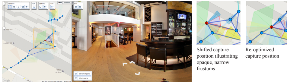
Figure 1: Left is a screenshot from the panorama moderation tool. Right is a zoomed selection of the map illustrating how the high-confidence links appear by shifting and re-optimizing a capture point. Note how the less likely links appear lighter and wider.
